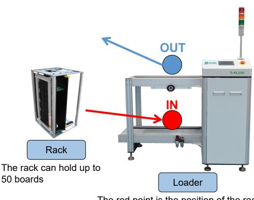
The loader automatically sends the board to S3010A, then S3010A will work, and the height and width of the track are matched and the width can be adjusted.
