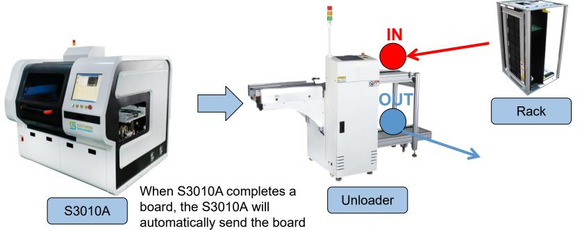
to unloader, and the height and width of the track are matched and the width can
